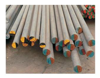
17-4 PH / 15-5 PH is a martensitic precipitation-hardening stainless steel that provides high strength, good corrosion resistance, good mechanical properties at temperatures up to 600°F (316°C) and good toughness in both the longitudinal and transverse directions in both base metal and welds. Short-time, low-temperature heat treatments minimize distortion and scaling. It may be used in the solution treated condition or heat treated to obtain a wide variety of properties.
